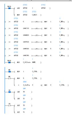
Figure 5.4 Programming case for multi-step setting and running
