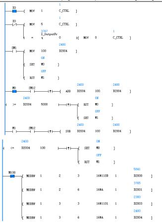
Figure 5.6 Programming case for RS485 communication
