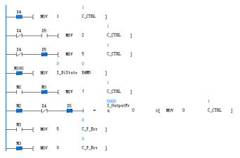
Figure 5.2 Programming case for terminal-based running/fault control
