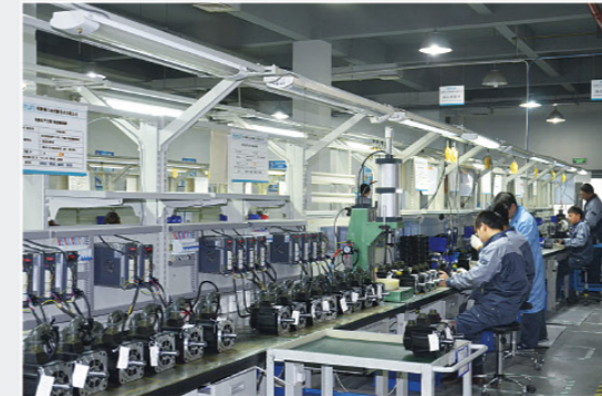
Servo Motor Production Line
